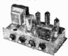
(11) The "Mono-Gram" A small Amplifier of genuine high quality performance producing up to 3 watts undistorted output. KIT OF PARTS £4.10.0. Built and tested £6.0.0 (C. & I. 3/6).
